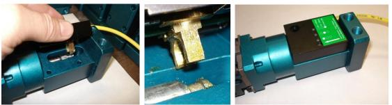
**Note:** Whenever any part of the gripper is replaced including pads the sensor will need to be recalibrated, see step J.
