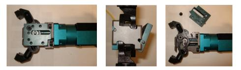
3) Remove jaw from gripper and flip gripper over to remove other jaw
