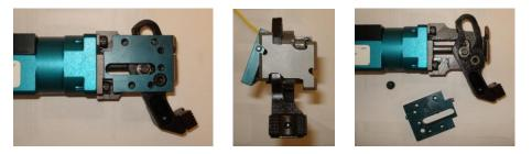
5) For lower jaws (11103 and 10151): Remove bushing from lower jaw using a small flat screwdriver or hex key and set aside for re-assembly. Lower jaw should be rotated completely down before removal. Lift up on front of jaw by pad so there is an angle between jaw and frame. Remove lower jaw from gripper.
