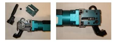
4) Remove SHCS and Schnorr washer from side plate. Rotate side plate up to about 45° angle and remove from gripper. Set SHCS and side plate aside for re-assembly.
