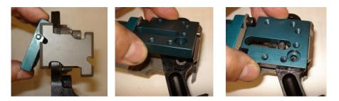
2) Add Schnorr washer to M5 X 12mm SHCS. Insert through side plate and into frame. Tighten M5 SHCS to **72in-Ib**.
