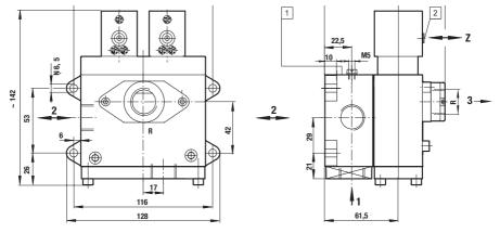
1 Flange surface for pressure switch or failure indicator unit
