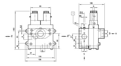
1 Flange surface for pressure switch or failure indicator unit
