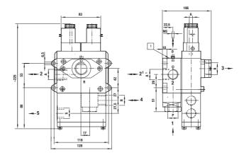
1 Flange surface for pressure switch or failure indicator unit
