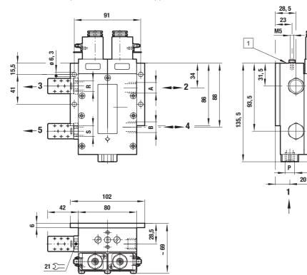
1 Flange surface for pressure switch or failure indicator unit
