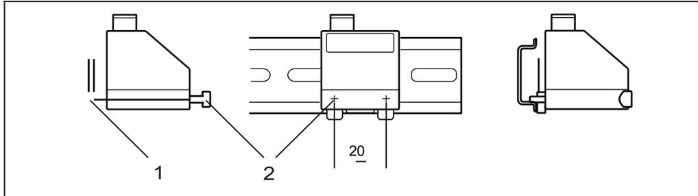
► Fix the mounting clip (1) with the M4 x 35 screws (2) to the flange.
