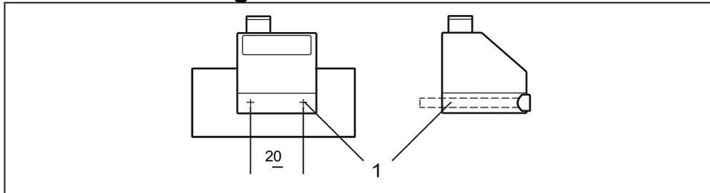
► Fix the unit with 2 M4 x 35 screws (1) (not included) to the rear panel. Maximum tightening torque: 2.5 Nm.
