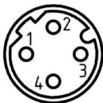
M12 / 4 pins / Female Connector / D-coded
