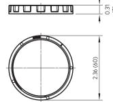
Recommended panel hole size: ø 55 mm ... 57 mm Panel thickness: 2 ... 6 mm
