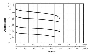
Inlet pressure: 145 psi (10 bar) Port size: 3/8", 40 µm element
