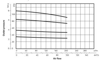
Inlet pressure: 145 psi (10 bar) Port size: 3/8", 5 µm element
