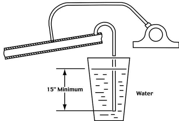
Figure 54. Checking manifold pressure with a water container.
