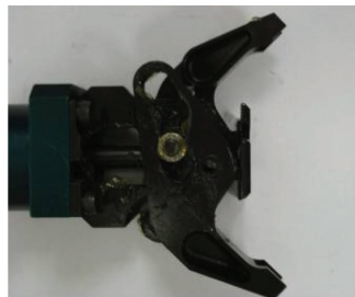
45° Open Jaw Angle Uses 45 degree (thin) stop
