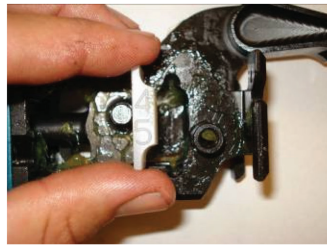
22° Open Jaw Angle Uses 22 degree (thick) stop
