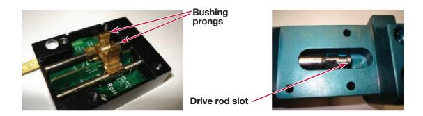
2. Apply Loctite 262 or equivalent to the three blind M4 tapped holes.
