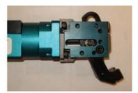
**4.** Remove SHCS and Schnorr washer from side plate. Rotate side plate up to about 45° angle and remove from gripper. Set SHCS and side plate aside for re-assembly.
