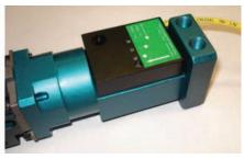
Note: Whenever any part of the gripper is replaced including pads the sensor will need to be recalibrated, see step J.
