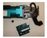
**5. For lower jaws (11103 and 10151):** Remove bushing from lower jaw using a small flat screwdriver or hex key and set aside for re-assembly. Lower jaw should be rotated completely down before removal. Lift up on front of jaw by pad so there is an angle between jaw and frame. Remove lower jaw from gripper.
