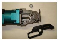
6. For lower jaws (11102): Remove lower jaw from gripper.
