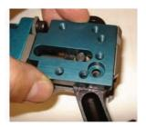
2. Add Schnorr washer to M5 X 12mm SHCS. Insert through side plate and into frame. Tighten M5 SHCS to 72in-lb.
