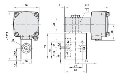
Solenoid optional turnable Working port 1/4 NPT
