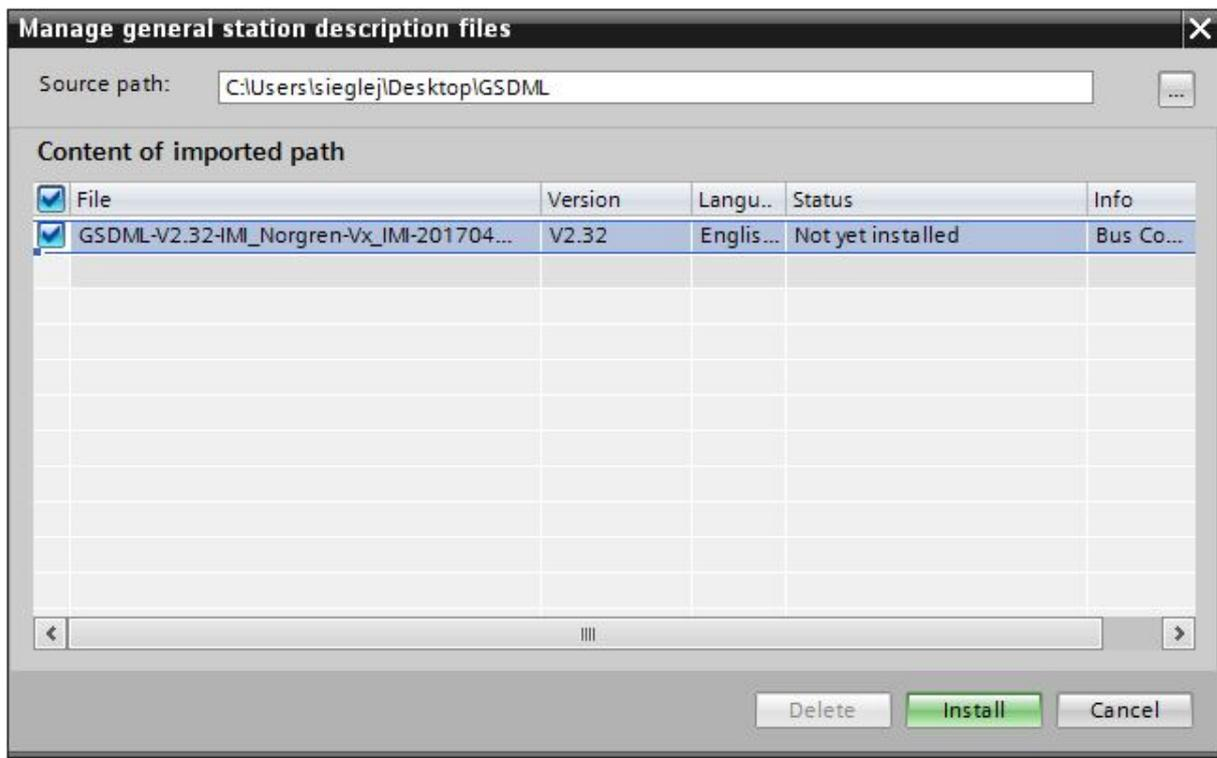
After the successful installation of the GSDML-file the VM10 is listed in the Hardware catalog.
