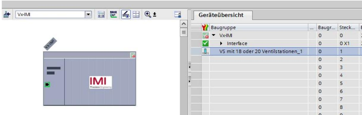
Double click the symbol to change into diagnostics view of the module. Highlight the “Diagnostic status” line to get detailed information about the pending module diagnostics
