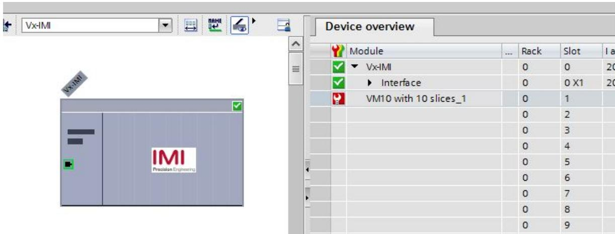
Double click the red symbol to change into diagnostics view of the module. Highlight the “Diagnostic status” line to get detailed information about the pending module diagnostics
