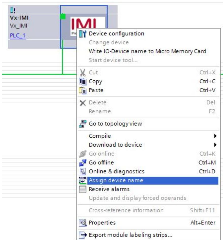
Enter a unique device name for the valve island in the “PROFINET device name” field. Push the “Assign name” button to assign the entered device name.
