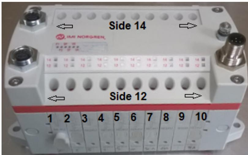
The illustration below shows the assignment for maximum configuration of 16 valve slices. For every valve two bits will be reserved – one bit for solenoid 14 and one bit for solenoid 12
