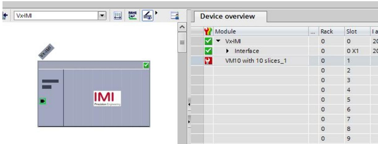
Double click the red symbol to change into diagnostics view of the module. The channel number and the error reason are shown in the “Channel diagnostics” table.
