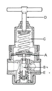
re against the diaphragm increases, causing the diaphragm to impress the adjusting spring until the load exerted by the gulated pressure equals the spring load. If there is no flow emand, this state of equilibrium will occur with the valve osed. If there is a flow demand, this state of equilibrium will occur with the valve open just the amount necessary to compente for the demand, thus maintaining the desired regulated ressure.
