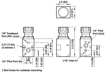
† Bolt holes for subbase mounting †† Air inlet for subbase mounting
