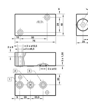
1 Inlet port 1 2 Outlet port 3 Inlet port 11
