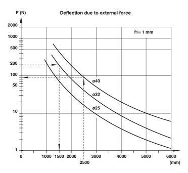
Cylinder  $\emptyset$  32 mm, stroke length 3500 mm, external load 200 N Maximum distance between supports = 1500 mm (see diagram). Therefore additional support is required.
