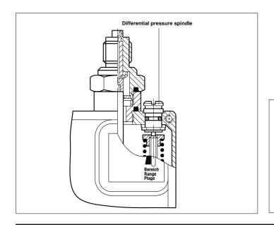
To set precise switching points a pressure gauge is required. (The pressure switch is a switching and regulating device and not a measuring instrument - even if it has a scale to assist in the setting). The setting can be changed at aby time, even during operation.
