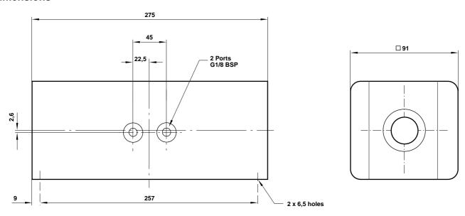
Dimensionally interchangeable with the M/2710
