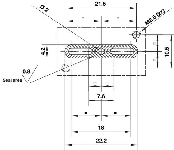
All solenoids are supplied with mounting screws and gasket,
