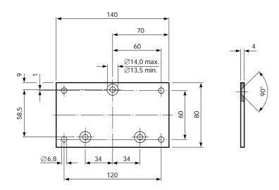
Mounting Plate for use when the valve cannot be mounted in the normal manner, reference QM/1149. Includes three M6 x 1 x 10 long bolts.
