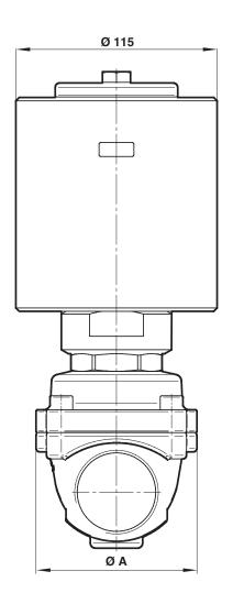
1 Solenoid rotatable 360° Socket turnable 4 x 90° (Socket included)
