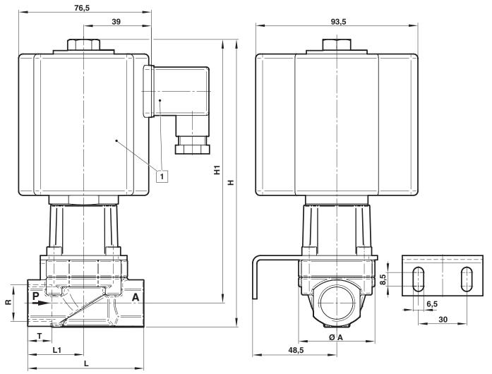
■ Solenoid rotatable 360° Socket turnable 4 x 90° (Socket included)
