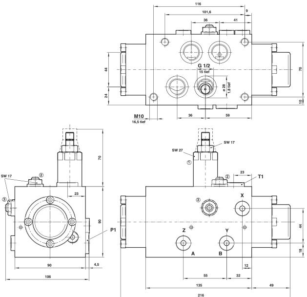
For subplate mounting 4 'O'-rings 23,47 x 2,62 (PRP-No. 119) are necessary. They are not included with valves without subplates (Part-No. 12 425 56).
