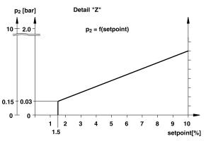
The valve function is activated as soon as the setpoint is ≥1,5%
