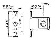
4314-52 - For use with W74 Use 6 mm (7/32") screws to mount bracket to wall.
