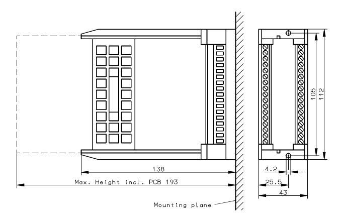
Installation of a bracket for the supporting rail increases max. height by 20 mm.
