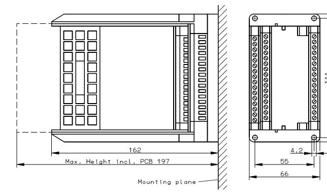
Installation of a bracket for the supporting rail increases max. height by 20 mm.
