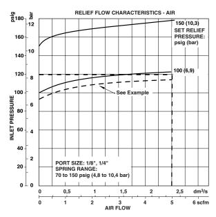
**EXAMPLE:** If your compressor delivers 5 scfm at 120 psig and your tank requires a working pressure of 90 psig, the relief valve must have a set pressure slightly higher than the 90 psig working pressure and be capable of flowing 5 scfm at 120 psig (or pressures less than 120 psig).
