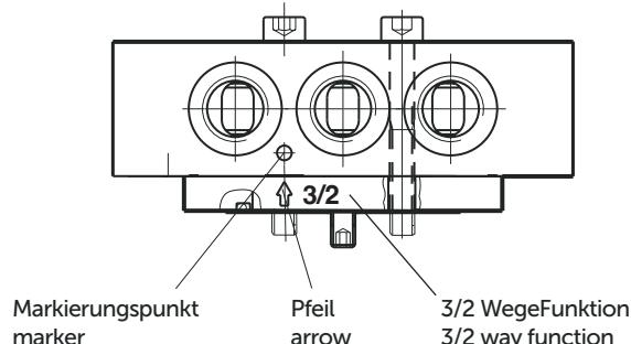
3/2 resp. 5/2 way function can be achieved just by swapping enclosed adapter plates. Make sure Marker and Arrow do match as shown on above drawing. Original mode of supply: 5/2 way function
