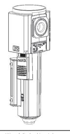
Bowl in unlocked postition (clip locking tab visible above LOCK). Bowl Bayonet tabs are in body. Turn bowl toward bowl alignment arrow on cover. Bowl will be in postion when lock clip snaps into body.
