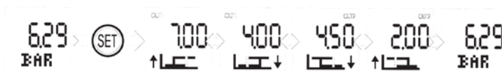
Picture 1: Switching OUT 1 in the standard mode with (n.o.), switching OUT 2 in the standard mode (n.c.)
