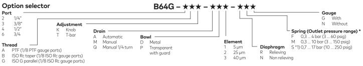
\* Outlet pressure can be adjusted to pressures in excess of, and less than, those specified. Do not use these units to control pressures outside of the specified ranges. \*1) Units with 17 bar (250 psig) adjustment range are available only with the T-bar adjustment, therefore substitute T at the 7th digit and S at the 12th position.
