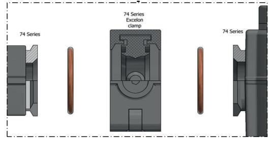
Shown above is the Excelon clamp 4314-51 (clamp with bracket 4314-52) connecting two Excelon 73/74 series products together (clamp footprint is 24.5mm wide)
