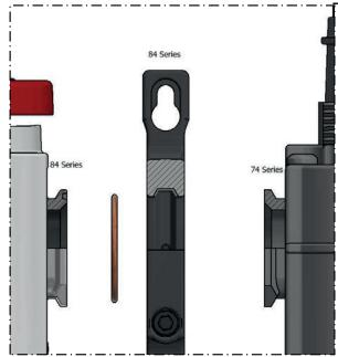
The inlet face of a 73/74 Excelon product has the same flat interface as the inlet face of a 84 series Excelon<sup>®</sup> Plus therefore an 84 series clamp, 840014-51KIT or clamp with bracket 840014-52KIT can be used as the connection system.
