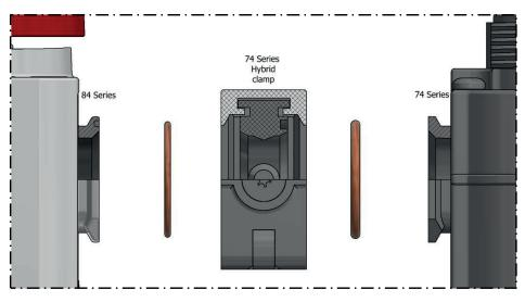
Both the hybrid clamp 840014-61 or hybrid clamp with bracket 840014-62 were designed to allow connection of the Excelon® Plus to Excelon series.
