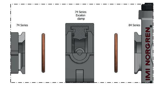
In the example above, with flow left to right, a 73/74 series Excelon product and an Excelon clamp 4314-51 (clamp with bracket 4314-52) connecting to an Excelon® Plus 84 series
