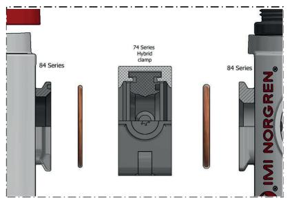
Both the hybrid clamp 840014-61 or hybrid clamp with bracket 840014-62 were designed to allow connection of the Excelon® Plus to Excelon series. But the clamp can also be used to accommodate connecting two Excelon® Plus 84 series products together (clamp footprint is 24.5mm wide)
