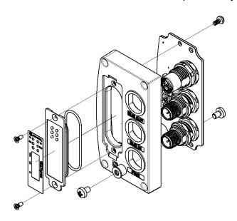
4. Remove circuit board 2 from bottom assembly
