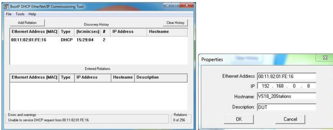
The IP Address settings are transferred into the “Discovery History” if they are valid and confirmed with the “OK” button. Pushing the “Enable BOOTP/DHCP” Button enables the IP Address assignment for the chosen entry. The VM10 valve island will appear with assigned IP Address in “Discovery History” list if address assignment was successful.
