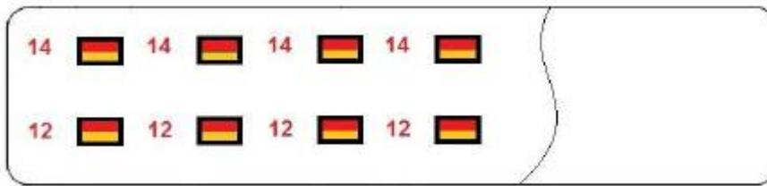
Each valve station has 2 separate status LEDs depending on its configuration, which indicate the control states “14” and “12” for the corresponding pilot valve solenoids.
