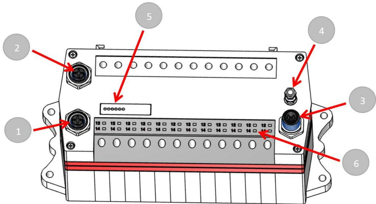
1. Port 1 bus connector for EtherNet/IP
