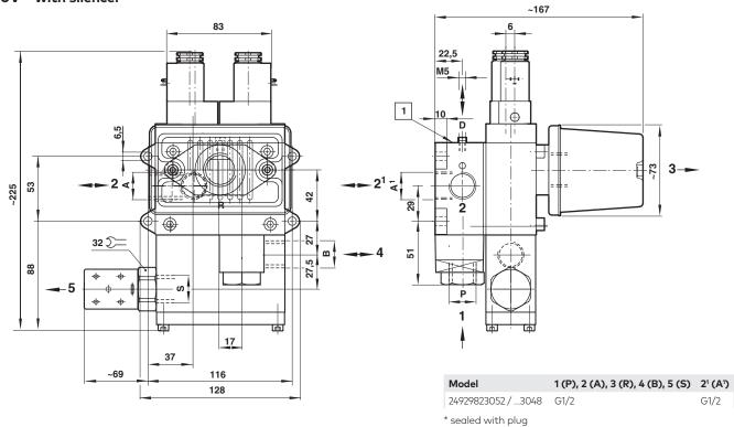
$\ensuremath{\boxed{1}}$  Mounting interface for pressure switch and failure indication module.
