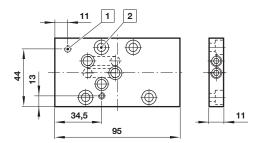
$\fill \ensuremath{ ext{1}}$  Two screws M4 x 50 mm deep to mount the VP50 onto the manifold  $\fill \ensuremath{ ext{2}}$  Four screws M6x16 mm deep to mount the manifold onto the iso subbase
