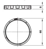
Recommended panel hole size: ø 55 mm ... 57 mm Panel thickness: 2 ... 6 mm
