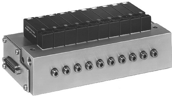
Valve terminal, Size 1, with multi-pin plug connector, IP 40, with ten 3/2 directional control valves
